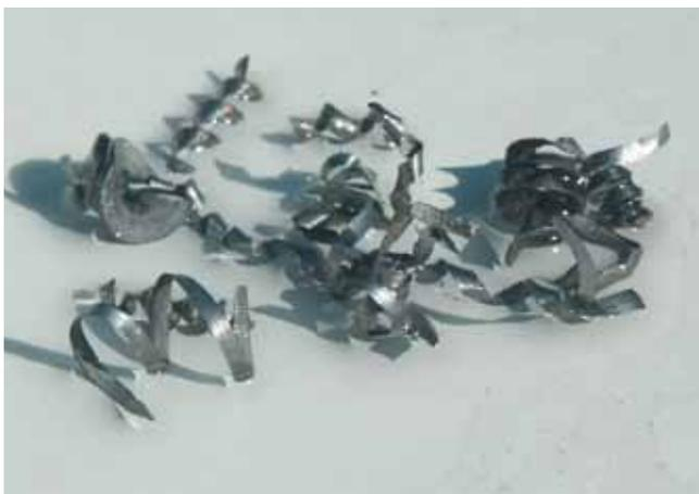
**Ensure all swarf (drill waste) is removed from the work area.**
